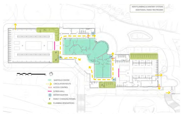
**Bathhouse Projects, Phase Two:** The second project phase should address rehabilitation of existing plumbing systems and the installation of new amenities such as drinking fountains and gender-neutral changing rooms.
